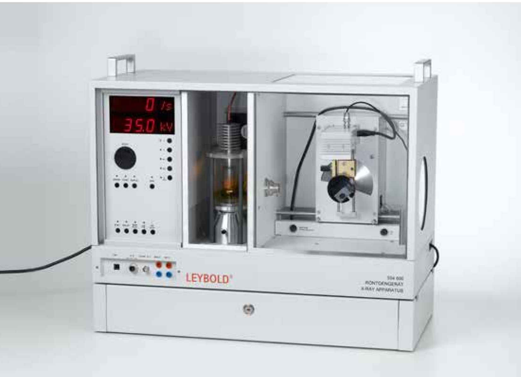
X-ray fluorescence analysis of chemical composition (C3.6.5.1)
